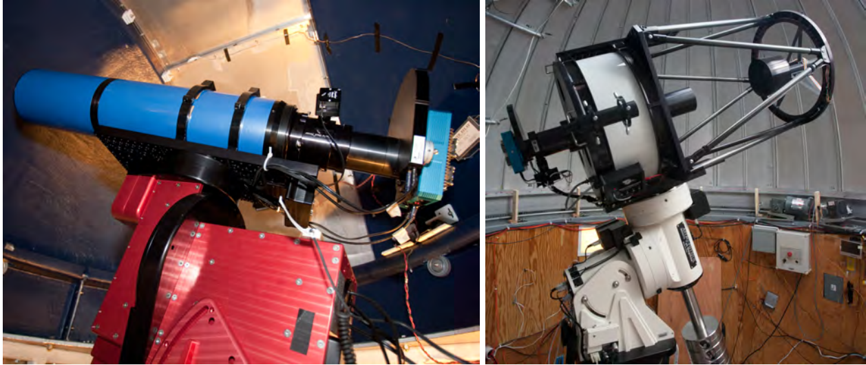
Figure 2. The 5.3 inch f/5.4 VYSOS-5 telescope built by Stellarmv Telescopes (left) in its dome at Mauna Loa Observatory. The 20 inch f/8.2 VYSOS-20 telescope built by RCOS (right).
