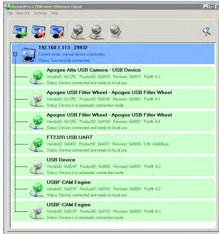
Figure 3. A screenshot of the client interface for the "USB over Ethernet" software. Available devices are shown with green symbols. In this case four available devices are shown: an Apogee Alta CCD camera, an Apogee filter wheel, our cloud sensor (which shows up as FT323R USB UART), and an SBIG guide CCD (which shows up as USBF-CAM Engine).
