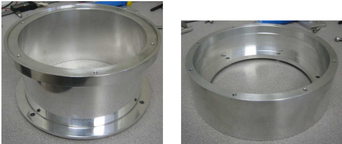
Fig. 2.— The two completed cryostat extenders. The first one is on the left, the second on the right.
