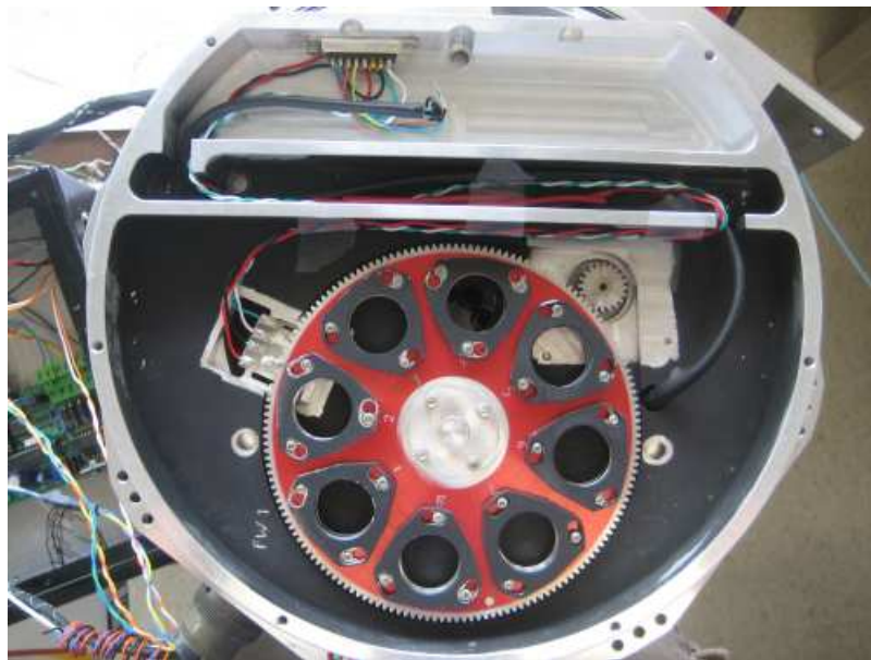
Fig. 4.— The filter wheel installation.
