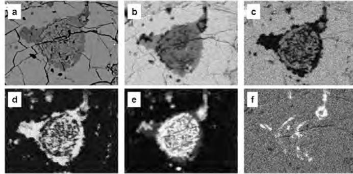
**Figure 12:** The element maps of MET00737 AOA#1. a: BSE image, b: Mg map, c: Fe map, d: Ca map, e: Al map, f: Na map. In this figure the Anorthite and Diopside dominate, and some spinel regions can be seen, and a well equilibrated matrix is again obvious.
