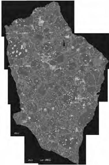
**Fig 5:** An example of an assembled meteorite map. This is the meteorite Y82094 thin section BSE map. This type of mapping was accomplished for all meteorites in the study.
