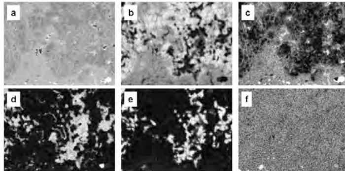
**Figure 14:** The element maps of Y82040 AOA#2. a: BSE image, b: Mg map, c: Fe map, d: Ca map, e: Al map, f: Na map. In this figure both the turtle shell pattern with Mg hot spots and Anorthite and Diopside regions can be seen.
