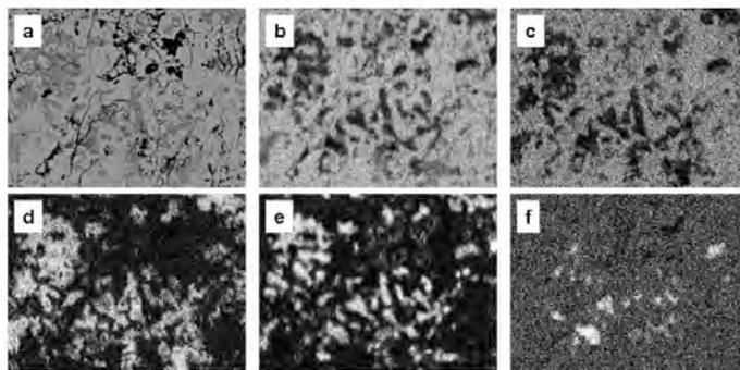
**Figure 11:** The element maps of MET00711 AOA#5. a: BSE image, b: Mg map, c: Fe map, d: Ca map, e: Al map, f: Na map. In this figure the Anorthite and Diopside dominate, and some spinel regions can be seen, and a well equilibrated matrix is again obvious.
