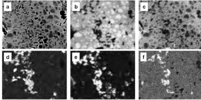
**Figure 9:** The element maps of A882094 AOA#3. a: BSE image, b: Mg map, c: Fe map, d: Ca map, e: Al map, f: Na map. The AOA has not yet equilibrated with the matrix as evidenced by the Mg hot spots in 9b, reinforcing the classification of a lesser altered meteorite. In addition, 9f demonstrates the attack of Na on the Anorthite.
