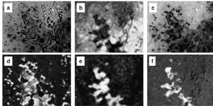
**Figure 13:** The element maps of QUE94716 AOA#2. a: BSE image, b: Mg map, c: Fe map, d: Ca map, e: Al map, f: Na map. In this figure both the turtle shell pattern and Anorthite and Diopside regions can be seen, in addition to the attack of Anorthite by Na.
