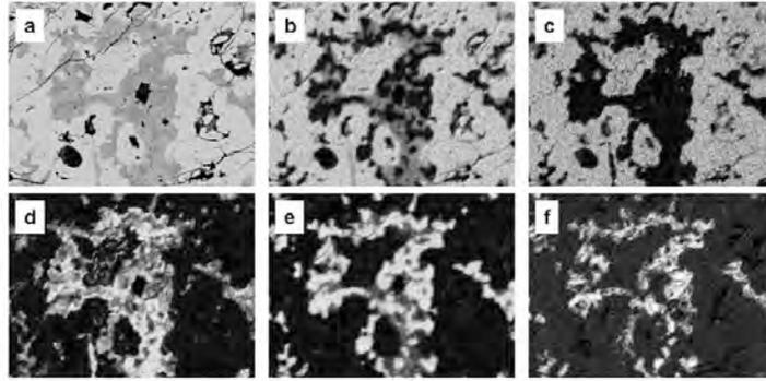
**Figure 15:** The element maps of ALH83108 AOA#5. a: BSE image, b: Mg map, c: Fe map, d: Ca map, e: Al map, f: Na map. A well-equilibrated AOA, as well as a good example of the Na attack on Anorthite.
