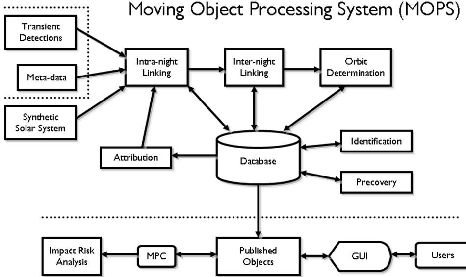
**Figure 3.** Moving Object Processing System concept of operations. Data in the upper left region surrounded by dotted lines is provided by the IPP. Systems below the horizontal dotted line are not part of the MOPS.
