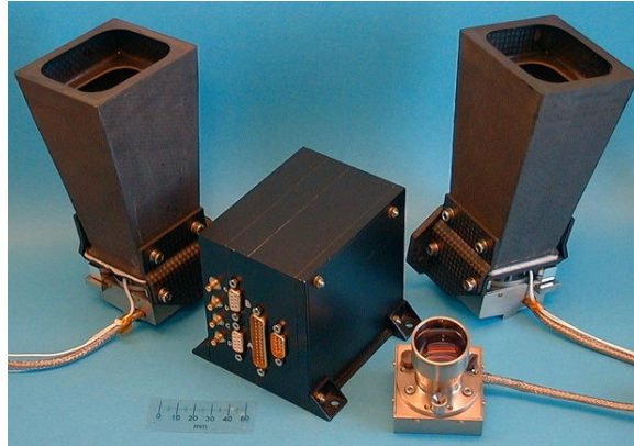
Fig. 1. The Advanced Stellar Compass Star-tracker
