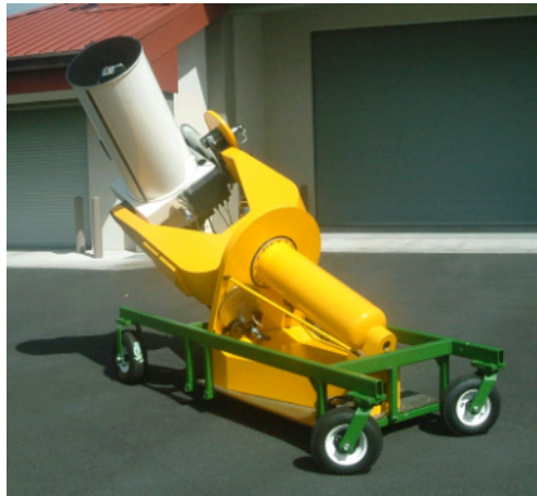
Fig. 2. The DFM 20" telescope mounted on the custom built cart in the car park of the IfA Hilo building
