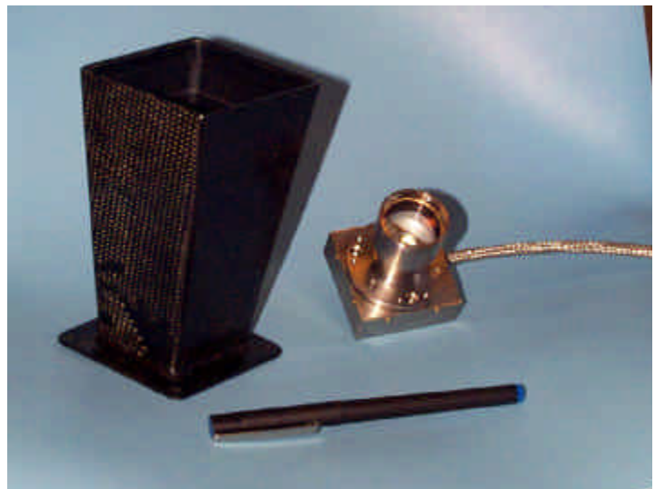
Figure 8, A camera unit next to a stray light suppression baffle.
