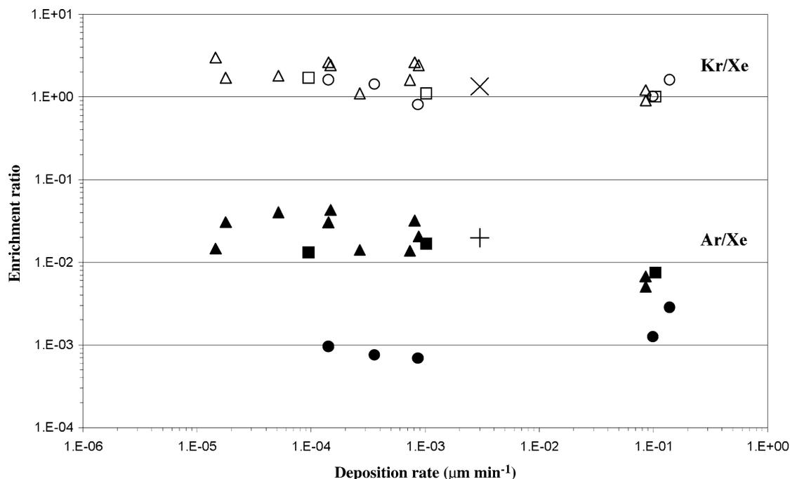
Fig. 3. Enrichment ratios (the ratio Kr/Xe or Ar/Xe trapped in the ice, divided by the ratio Kr/Xe or Ar/Xe in the gas mixture deposited together with water vapor on the cold plate) as a function of deposition rate: Kr/Xe in water ice deposited at 50 K (○), 27 K (△), and 22 K (□); Ar/Xe in water ice deposited at 50 K (●), 27 K (▲), and 22 K (■). We marked also the enrichment ratios in Earth's atmosphere, Kr/Xe (×) and Ar/Xe (+), which fit well the experimental values.
